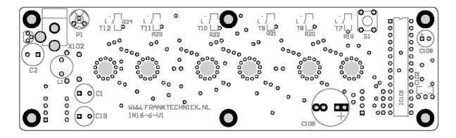
Some parts go at the bottom. Note the orientation of the 5V regulator near the DC input connector. Also take care mounting the capacitors, placing them in the right direction (polarity). The square hole indicates the positive lead of the capacitor. It may be wise to mount S1 a few millimeters above the pcb, so that the plastic extender sticks a little bit through the bottom plate.
