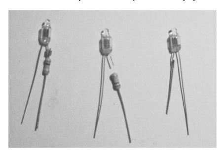
Cut away the resistor. Try to cut away the copper, leaving as much wire as possible. I often manage to bend the crimp open. Find a piece of stiff wire, and make the short leg longer. Now you can feed the wires through the plastic standoff, and mount it on the PCB. Do not solder for too long, or the wire may run too hot and unsolder itself from the neon lamp. Pull the lamp gently to check if it actually is still connected inside the plastic standoff.
