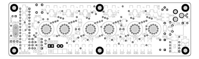
This picture shows which parts should be fitted on the top.
