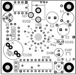
The transistors are mounted in a circle, on the bottom side. Also take care mounting the capacitors, placing them in the right direction (polarity). The long leg of a capacitor should go into the square hole.
